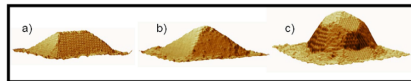
Figure 1: High resolution ultra-high vacuum scanning tunneling microscope (STM) images showing a) a hut cluster ( 50 \times 32 \times 3 \text{ nm}^3 ), b) a pyramid ( 50 \times 50 \times 7 \text{ nm}^3 ) and c) a dome island ( 50 \times 50 \times 10 \text{ nm}^3 ), formed after the deposition of Ge onto a Si(001) surface [8]. The size of the islands can be adjusted by the growth parameters.
